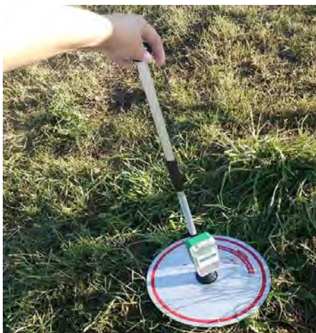
Electronic rising plate meter used to collect pasture herbage mass during the grazing season
