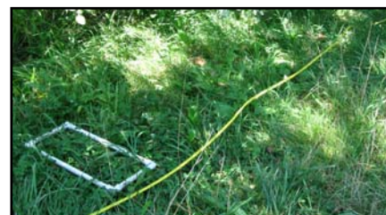
Fig. 11: Daubenmire PVC Frame and Tape Measure along a transect.
